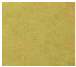
Machine Trowel Finish
